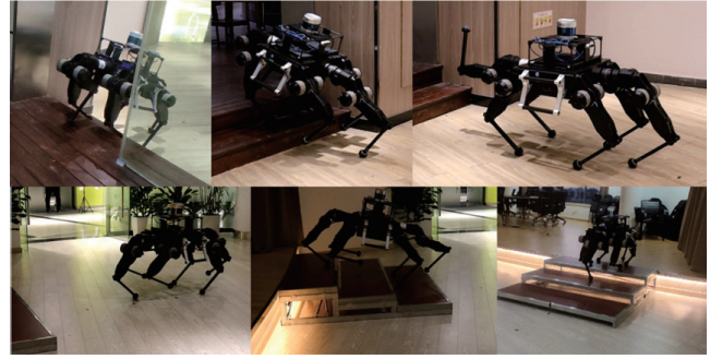
Fig. 8. Video screenshots of Qingzhui long-range locomotion under CapPlanner's control
