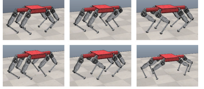
Fig. 3. The Topologies of Qingzhui Robot. The topologies from left to right are Nominal, Hind-Bend, Front-Bend, Hind-1-Bend, Front-1-Bend, Split-Up
